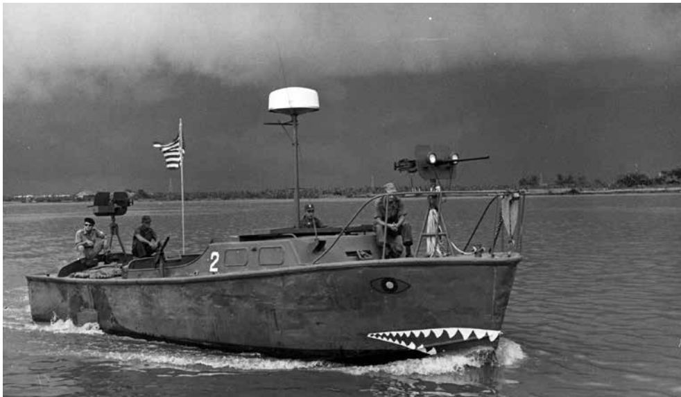
LCPL on the Saigon River, October 1965. These 36-foot-long patrol boats provided security for the Saigon shipping channel prior to the arrival of the PBRs.
