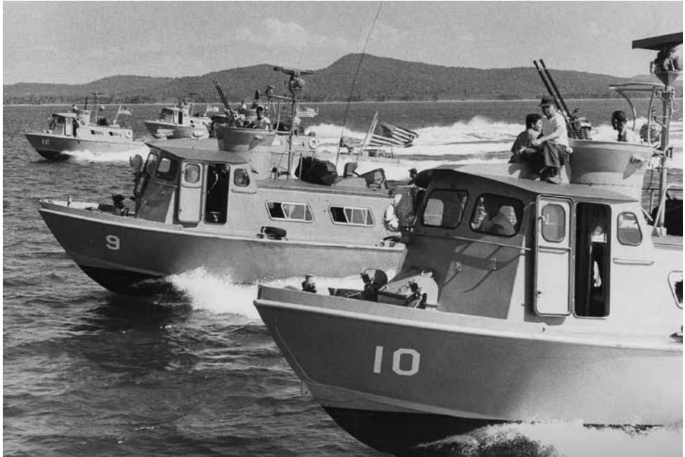
PCF Swift boats of Division 101 underway in the Gulf of Thailand off Phu Quoc Island. The Swift boat’s shallow 3.5-foot draft and high speed of 28 knots made it an ideal craft for coastal patrol in Vietnam, December 1965.
