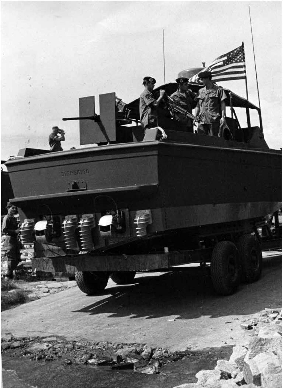
This late-model Mark I boat (PBR-130) on the trailer features four finned underwater exhaust pipes for quiet running and two water jet nozzles with gates, shown here in the up position for forward motion. If they were in the down position, covering the nozzle discharge opening, the closed gate would cause water to shoot under the boat, resulting in reversing the boat's motion.
