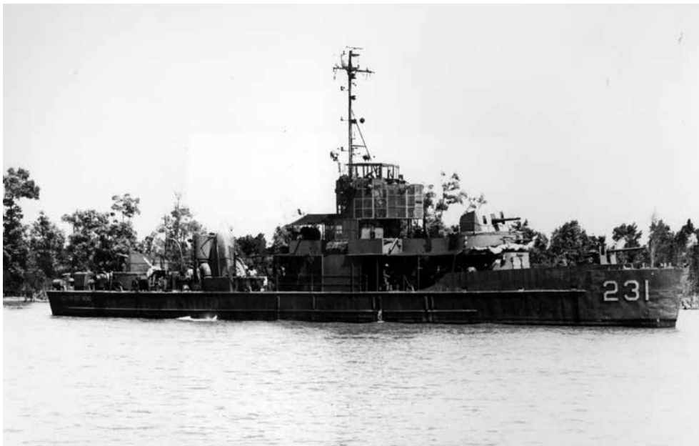
Nguyen Doc Bong (HQ-231), a 250-foot Vietnam Navy gunboat. Crewed by six officers and 65 enlisted sailors, the ship could reach speeds of up to 16.5 knots, circa later 1960s. In World War II, the boat served with the U.S. Navy as LSSL-129.
