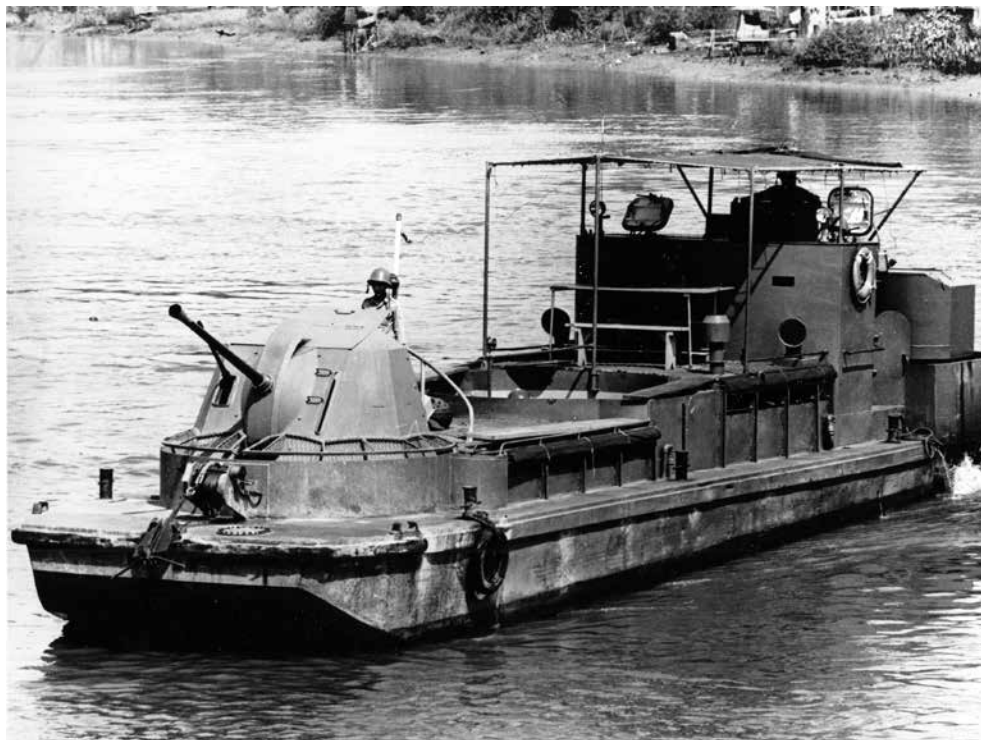
A Vietnamese Navy LCM monitor conversion armed with a .50-caliber machine gun, 20mm and 40mm cannons, and an 81mm mortar, 31 August 1964.
