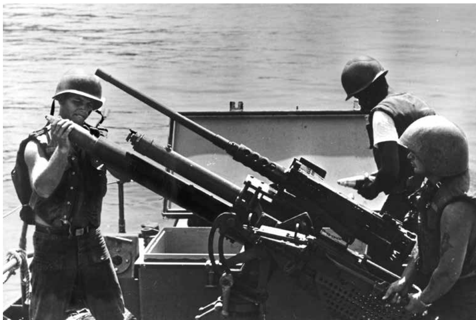
The mortar crew of PCF-54, Coastal Division 14, based at Cam Ranh Bay, prepares to fire a Mark II 81mm mortar. A .50-caliber machine gun is mounted on top of the mortar, 6 April 1967.
